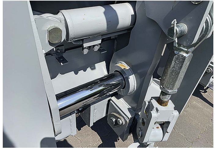
The guide tubes are chrome-plated and have maintenance-free bushes. The paintwork on out test frame was poor.
