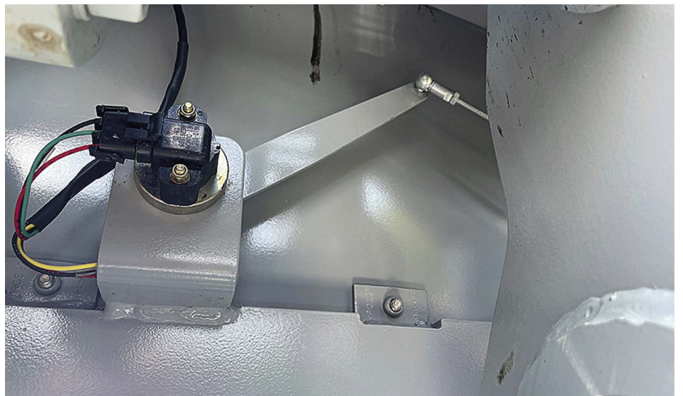
A John Deere position sensor monitors the side-shift position with the latter showing up on the tractor's in-cab display.
