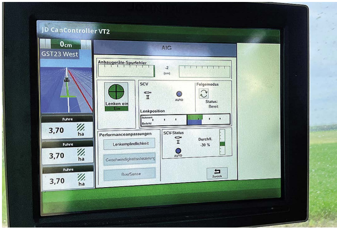
Our test John Deere control unit displayed tracking errors and target position of the side-shift platform. The latter was worked via one of the tractor spools.
