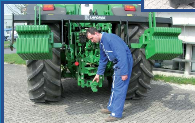
FLEXIMASS® rear with EASYMASS® weights remains stable when parked
