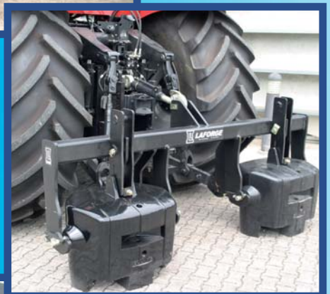
FLEXIMASS® rear with EASYMASS® weights remains stable when parked
